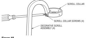
3. Slide the assembled decorative scroll over the 12" downrod and position each scroll leg on the decorative light kit ring (Figure 19). Secure each of the four decorative scroll legs using four #8-32 x 15mm flat head screws (supplied).
